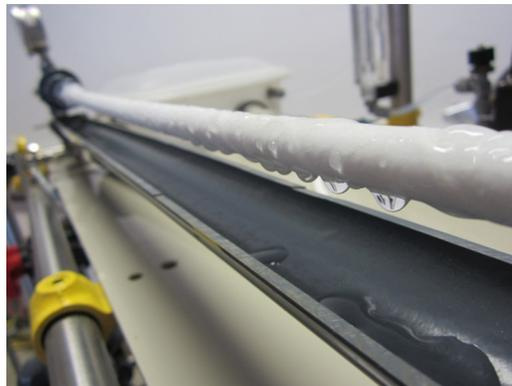
**Picture 1:** Open tubular membrane with dike
